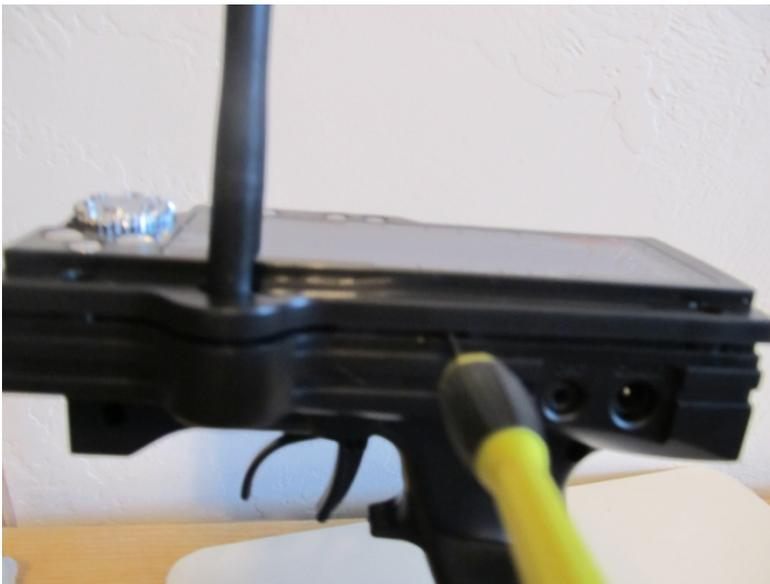
however this may lead to worse damage. To disengage the plastic latches use a small flat head and insert in the places shown on the picture and gently pull up on the cover...on the front side its located near the diagonal on the screen pop out, and the back side is located directly across
